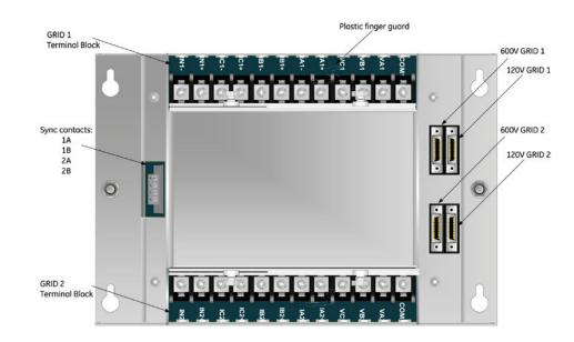
The interface module supports direct connect up to 750 VAC RMS so voltage transformers (PTs) are optional for low voltage power systems. Current transformers (CTs) are required for all current measurements.
